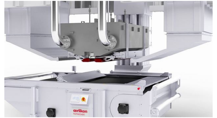
The hycuTEC process easily achieves filtration efficiencies in excess of 99.99% in the case of typical filter media
