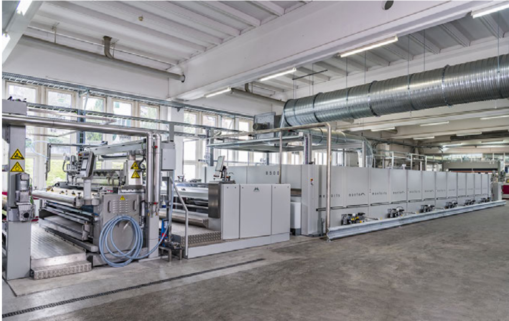
Monforts Montex stenters and coating units are the industry standard for the fabric finishing industry.
