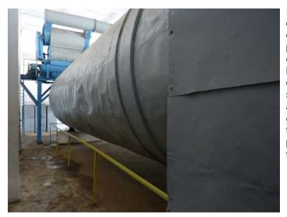
In the gin the seed cotton is dried in very large rotating drums, though which air is passed, the temperature depending on the measured humidity, rather like a clothes drier, but on larger scale A system that the Committee applauds as a manner to gentle dry without damaging the cotton fiber. After this process the cotton travels first to a horizontal cleaner, unique
